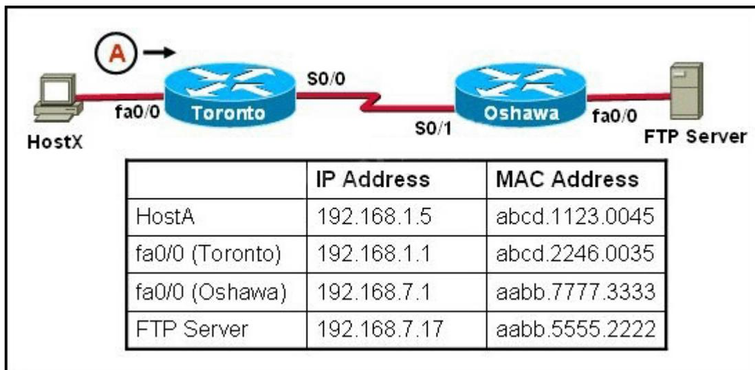
HostX is transferring a file to the FTP server. Point A represents the frame as it goes toward the Toronto router.
