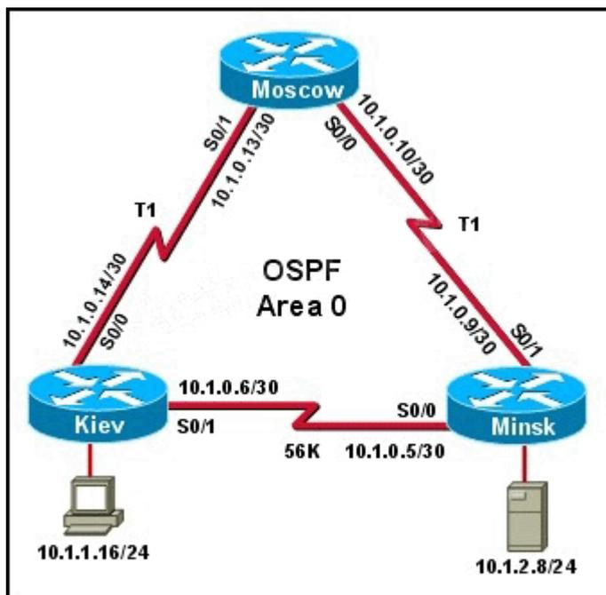
The host in Kiev sends a request for an HTML document to the server in Minsk. What will be the source IP address of the packet as it leaves the Kiev router?
