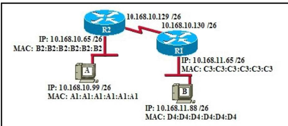
If host A sends an IP packet to host B, what will the source physical address be in the frame when it reaches host B?
