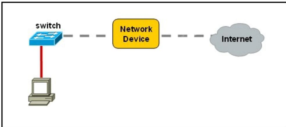
A network device needs to be installed in the place of the icon labeled Network Device to accommodate a leased line attachment to the Internet.
